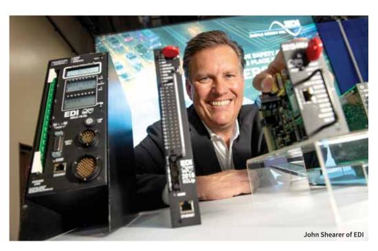
range of intersection types and operations. It also offers a significant safety upgrade, for both drivers and technicians. Its CMU current load monitoring detects a dark approach immediately, and its majority low-voltage components make installation and maintenance much safer. Add to that true LED compatibility that can support the latest ultra-low-power LED signals, and EDI says it's no surprise the ATC standard has had the fastest adoption rate of any cabinet standard in history.
